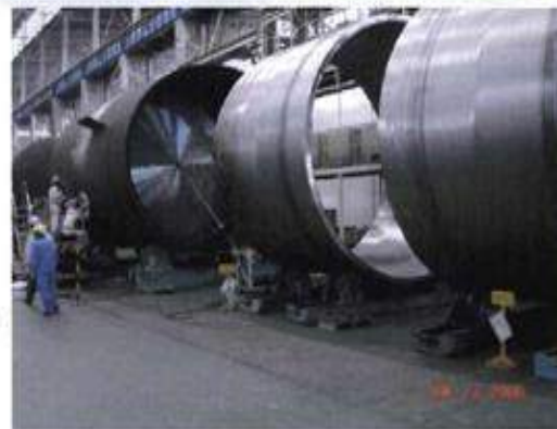
S/G 3A Lower and Middle Shell S/G 2A Balance Ring, Extension Ring, & Tubesheet
